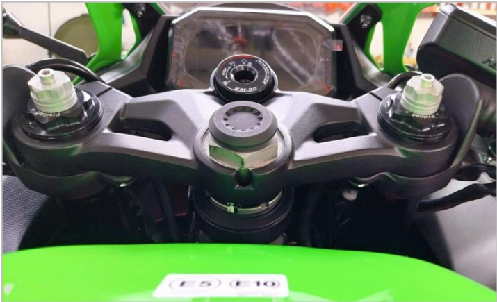
F20K cartridge fork kit / quad-valve asymmetric system
