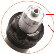
F20K cartridge fork kit / quad-valve asymmetric system
